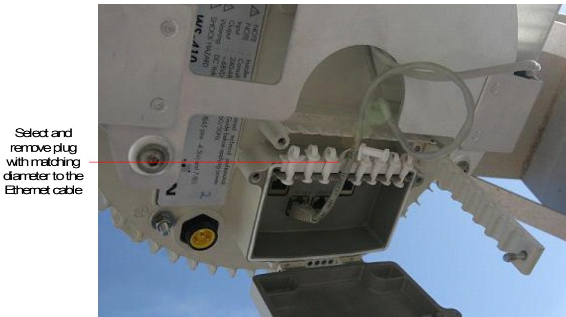
Figure 3.21. Removing the Plug Matching the Diameter of the Cable
