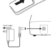
**2** Set the charger on a desk or table, then set the handset in the charger with the keypad facing forward.
