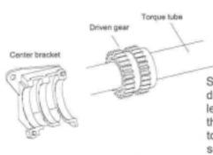
Slide the new Center Bracket onto the driven gear from underneath. Next, level the torque tube with the top of the door and secure the Center Bracket to the header with (1) 1/4 x 1 1/2" lag screw in the bottom hole as shown.
