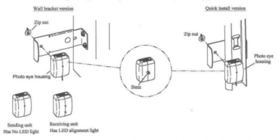
Uncoil wires from photoelectric sensors and route wire up garage wall and along door header towards right side of power head. Route wires behind torque tube and tack wires in place with insulated staples (not supplied).
