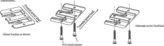
Align two snap posts on light fixture with two corresponding slots in fixture bracket, making sure interface socket is facing towards power head as shown. Slide light fixture into fixture bracket as shown until light fixture snaps into place.
