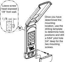
Insert screw into the upper pilot hole leaving the head of the screw exposed about 1/8" from the wall. Slide and lock the back keyhole slot over the exposed screw and position the unit vertically. Remove battery door and battery. Insert the lower screw and tighten. Replace battery and battery door.
