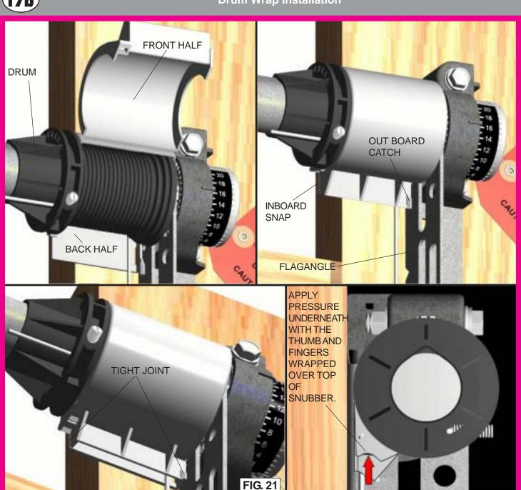
Locate right hand drum wrap. Slide back half of the drum wrap behind drum placing the right end wall between the drum and flag angle. Close front half of the drum wrap around drum, engage inboard snap and press firmly until a distinct snap is felt. Outboard catch must be engaged as shown. Confirm both snap and catch are fully engaged by lightly tugging against them. Repeat for the left side.
