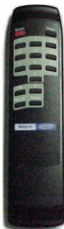
Figure 3-3 IR Remote Control. Use the remote within 12 inches of the display to set unit prices, blend ratios and fueling point ID, read totals, view error codes and other dispenser diagnostic functions.
