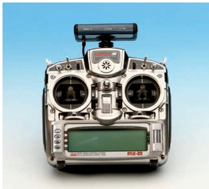
weatronic 2.4 Dual FHSS transmitter module on Graupner/JR transmitter MX22
