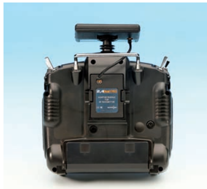
weatronic 2.4 Dual FHSS transmitter module on Graupner/JR transmitter MX22
