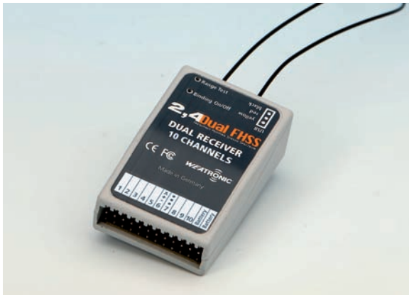
Dual Receiver 2.4 Dual FHSS micro 12 (left), 12 channel transmitter module (right)
