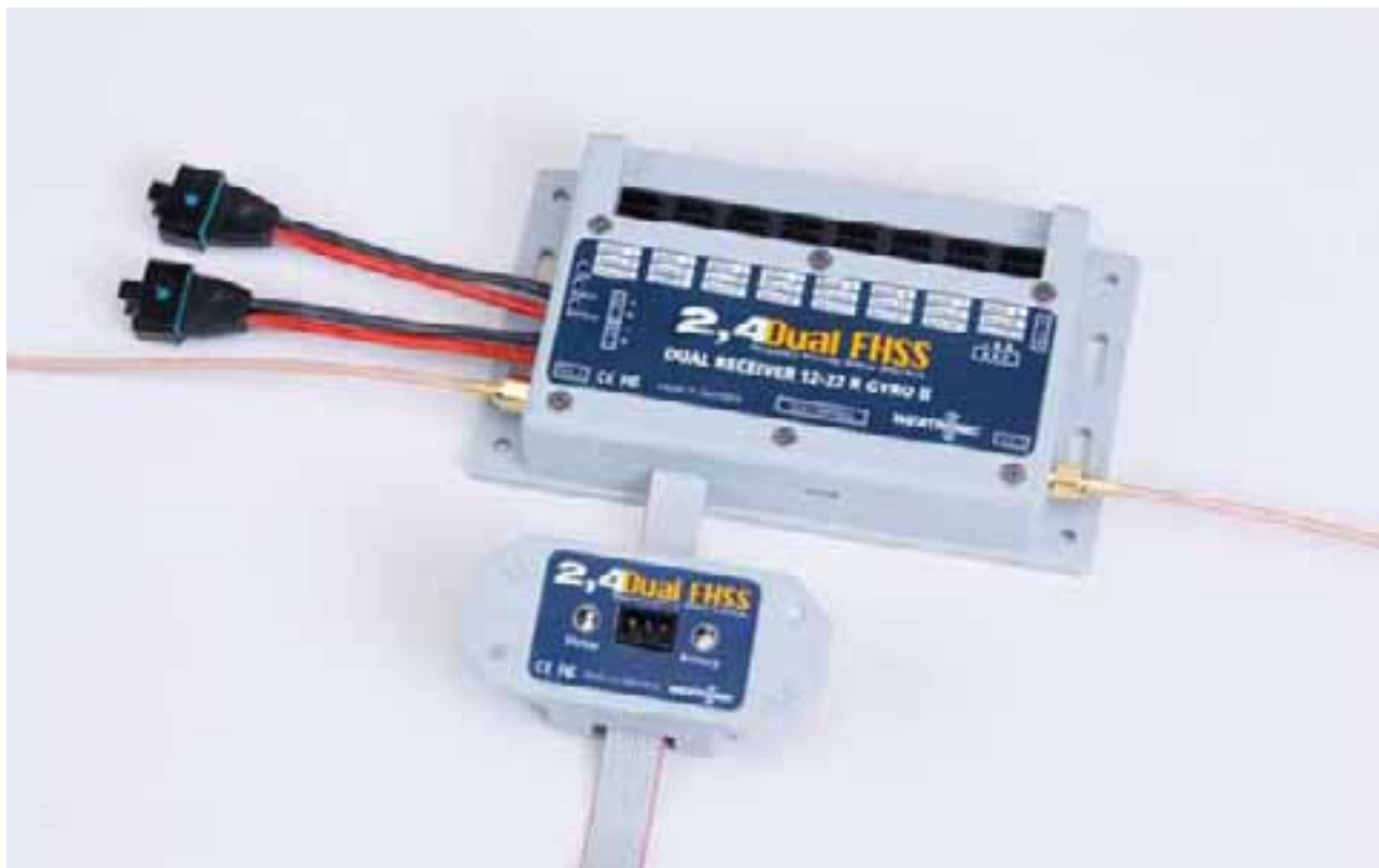
Dual Receiver 2.4 Dual FHSS 12-22 R Gyro II with electronic switch board
