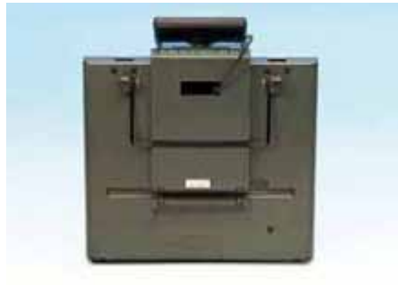
Connecting cable fed out through the visibility window hole on a Multiplex Profi MC 4000 transmitter
