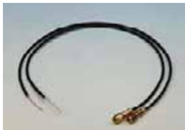
Original antennas with SMA type connectors
