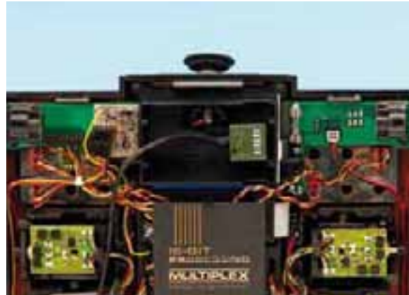
Opened Multiplex Profi MC 4000 transmitter showing the adapter module fitted
