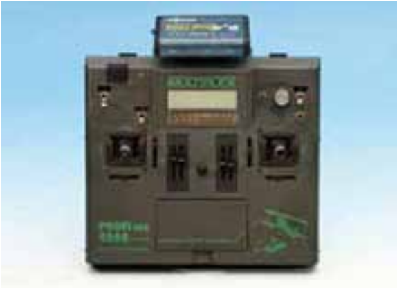
Weatronic 2.4 Dual FHSS transmitter module fitted to a Multiplex Profi MC 4000 transmitter
