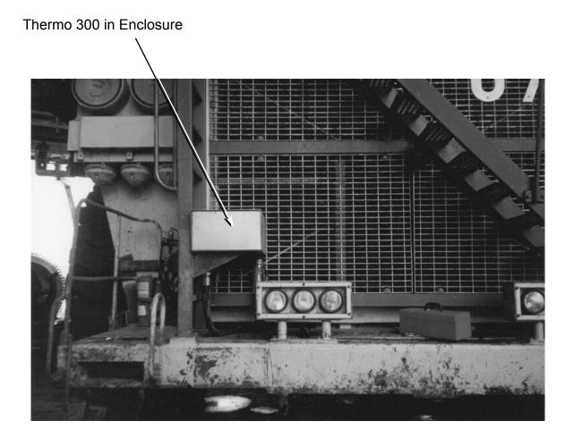
Fig. 5-4: Example of Heater Installation
