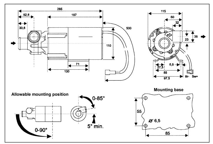
Fig. 4-3 Coolant Circulation Pump U4852 Dimensions
