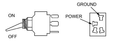
Fig. 5-7: On/Off Switch
