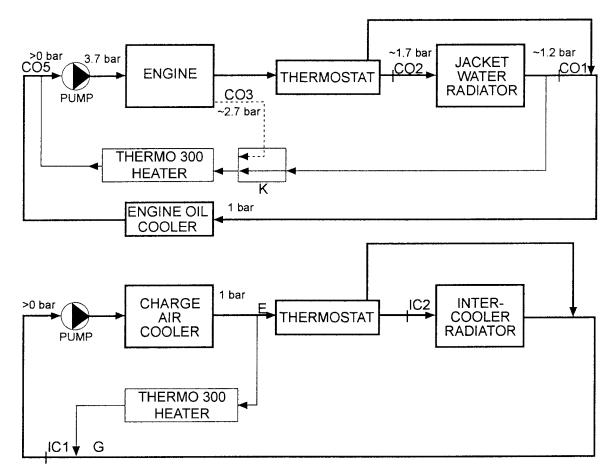
Fig. 5-1: Supplemental Heating Schematic
