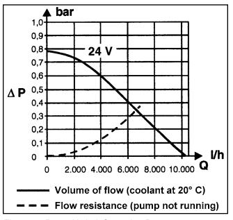
Fig. 4-4 Pump U4852 Operating Data
