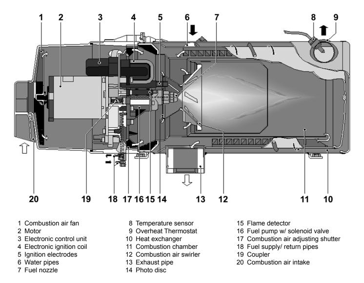
Fig. 2-1: Major Components of the Thermo 300 Coolant Heater
