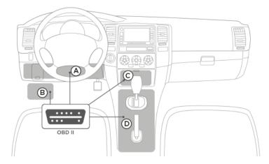
Refer to the manual of your vehicle. In many vehicles you can find the OBD-II port in the footwell (A), close to the fuse box (B), beneath the dashboard (C), or in the centre console (D).
