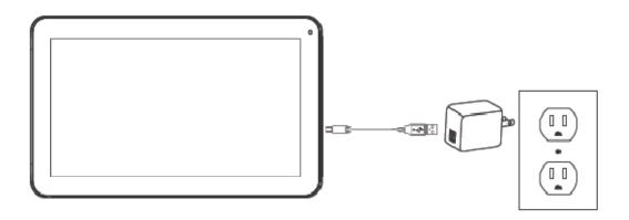
Plug the charger into a power outlet. The screen will display a flashing battery symbol for a few seconds to show that the battery is charging. Keep the battery on charge for 6 to 8 hours to make sure that it is fully charged.
