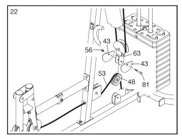
23. Route the Low Cable (53) under a Thick Pulley (48).
