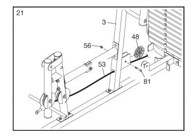
22. Route the Low Cable (53) over a Thick Pulley (48).
