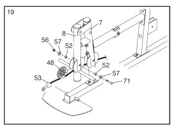
20. Attach a Thick Pulley (48) inside the Front Leg (7), above the Low Cable (53), with an M10 x 67mm Bolt (71), two M10 Washers (57), two 13mm Spacers (52), and an M10 Locknut (56).
