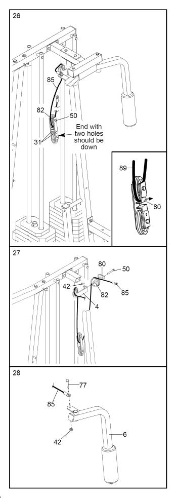
29. Note: The 3 1/2" Pulley (82) in this step is pre-assembled. It is shown removed for easier part identification.
