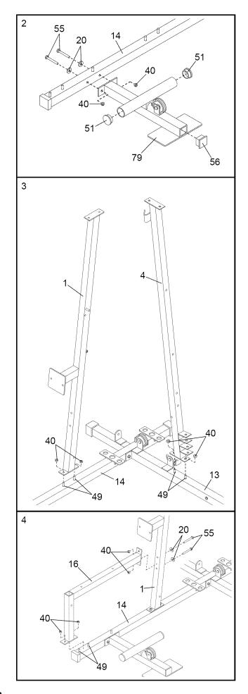
Slide the Front Seat Frame (8) onto the indicated 5/16" x 2 1/2" Carriage Bolts (49) in the Press Base (13). Partially tighten a 5/16" Nylon Locknut (40) onto each Carriage Bolt. Do not fully tighten the Nylon Locknuts.
