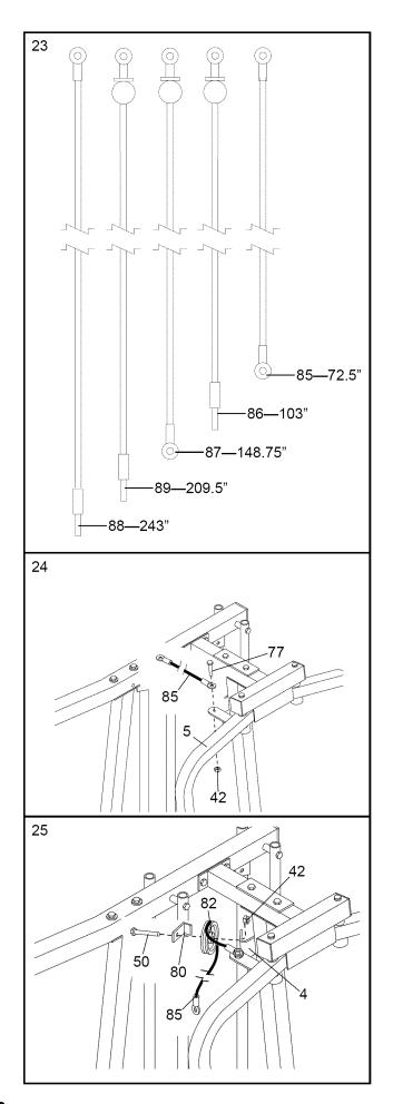
Route the Butterfly Cable (85) under the indicated 3 1/2" Pulley (82). The end of the Pulley Plates (31) with two holes should be downward. Refer to the inset drawing. **Be sure that the Cable is between the Cable Trap** (80) and the Pulley, and that the Cable Trap is positioned to hold the Cable in place.
