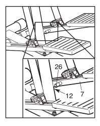
between the Reed Switch and the Magnet. Make sure that the Magnet will not hit the Reed Switch when the Right Pedal Leg is moved. Repeat until the console displays correct feedback.
