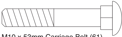
M10 x 53mm Carriage Bolt (61)
