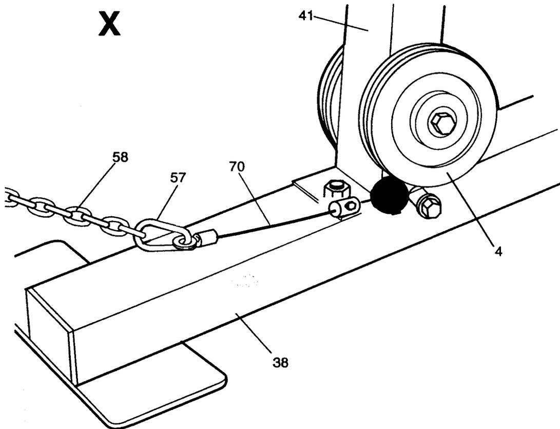
Note: It is important that cables must be kept in tension at all times. For correct operation the cables must be tensioned. To adjust, select maximum stack weight, loosen bolt in base ferrule, slide ferrule towards pulley (4). When all cable slack has been removed, securely tighten ferrule bolt. Damage will occur if this is not carried out.
