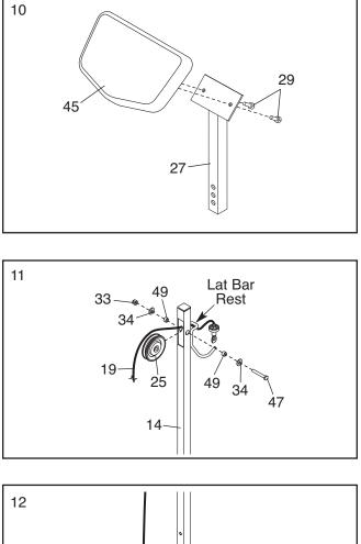
11. Route the Cable (19) through the Lat Tower (14) and over the Pulley (25). Make sure that the Cable is under the lat bar rest. Attach the Pulley inside the Lat Tower with an M10 x 50mm Bolt (47), two M10 Washers (34), two 10mm Large Spacers (49), and an M10 Locknut (33).
