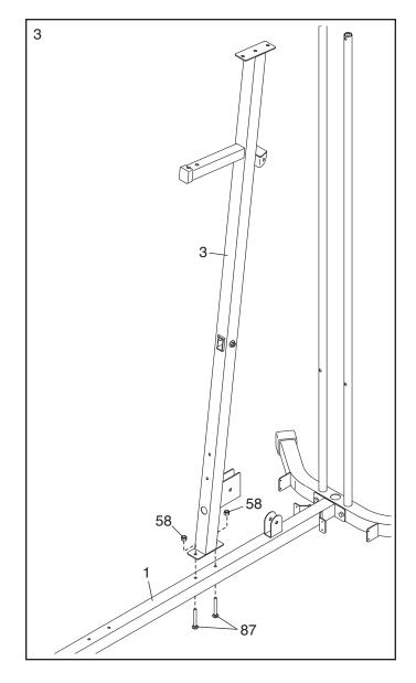
4. Attach the Front Leg (7) to the Base (1) with two M8 x 63mm Carriage Bolts (87) and two M8 Locknuts (58). **Do not tighten the Locknuts** yet.
