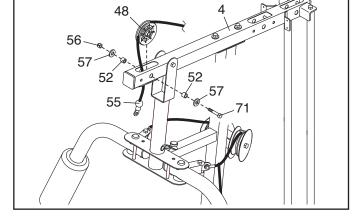
26. Route the High Cable (55) over a Thin Pulley (47) and downward through the Top Frame (4).
