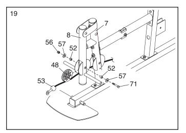
20. Attach a Thick Pulley (48) inside the Front Leg (7), above the Low Cable (53), with an M10 x 67mm Bolt (71), two M10 Washers (57), two 13mm Spacers (52), and an M10 Locknut (56).
