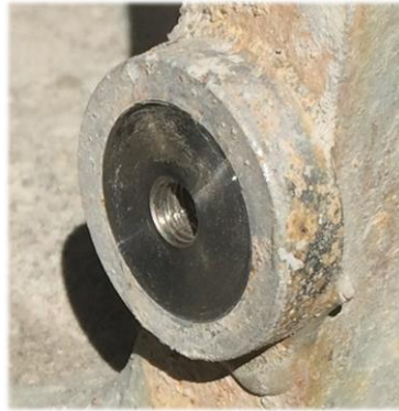
Figure 13-4 Slurry pump - Mounting pump adhesively bonded to pump
