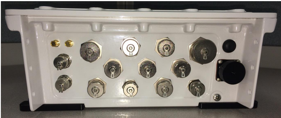
Figure 6-3 MPM connector view - protective caps installed
