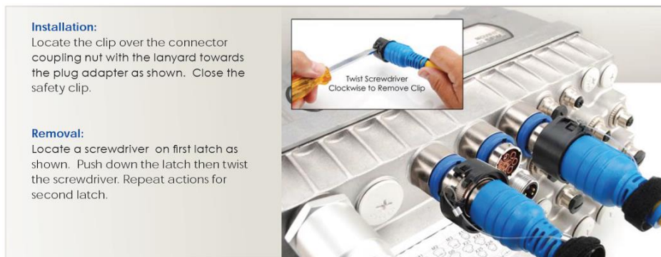
Figure 12-1 Installation of Locking Clips
