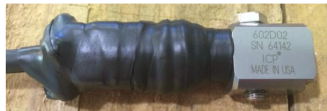
Figure 13-5 Uni-axial accelerometer with connector and protective tape applied
