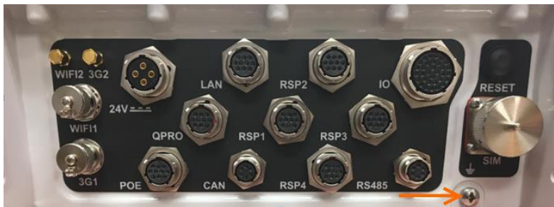
Figure 6-14 Location of Protective Earth Grounding on MPM
