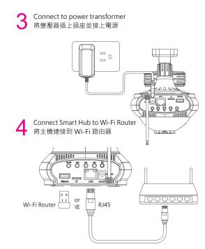
3 minutes to activate after power on then the LED indicator turns to blue 啟動電源3分鐘後 LED 指示燈變成藍色
