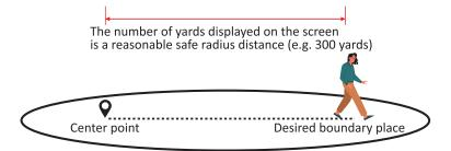
• Please leave the center point after both center point and maximum radius distance 999 yards are set up,then walk to the boundary where you want to stop at, now the distance shown on the screen the yards away from the center point, and this yard is the most reasonable safe radius distance
