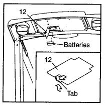
two batteries into the console. Make sure that the negative (-) ends of the batteries are touching the springs. Close the battery cover, push up on the tab, and then push the tab forward as shown in the inset drawing. Make sure that the tab locks into place.
