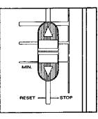
Next, slowly slide the speed control up until the walking belt begins to move at slow speed. Carefully step onto the walking belt and begin walking. Change the speed of the walking belt as desired by sliding the speed control.
