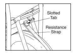
resistance strap, first turn the resistance knob counterclockwise to the lowest setting. Next, locate the slotted tab on the front of the exercise bike. Grip the longest part of the resistance strap underneath the slotted tab and pull it towards the slot. When a little slack is created, pull the end of the resistance strap tight. Turn the crank for a moment to make sure that there is not too much resistance.
