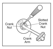
screwdriver in one of the slots in the slotted crank nut. Lightly tap the screwdriver with a hammer to turn the slotted crank nut counterclockwise until the arms are no longer loose. **Do not overtighten the slotted crank nut.** When the slotted crank nut is properly tightened, retighten the crank nut.
