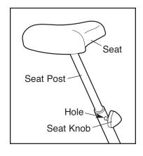
Next, align a different hole in the seat post with the indicated hole in the frame, and insert the seat knob into the frame and the seat post. Make sure to insert the seat knob into the seat post; do not insert the seat knob under the seat post. Tighten the seat knob into the frame.
