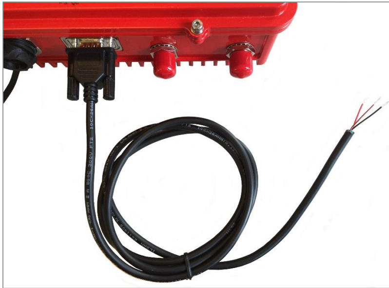
Figure 5-6: Alarm Relay Cable Connected to Repeater
