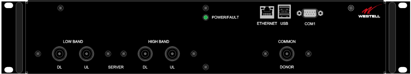
Figure E-16: Dual-band D1:S4 Port Configuration
