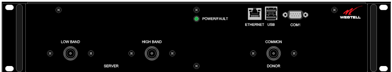
Figure E-10: Dual-band D1:D2 Port Configuration
