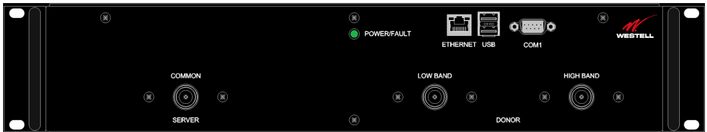
Figure E-9: Dual-band D2:D1 Port Configuration
