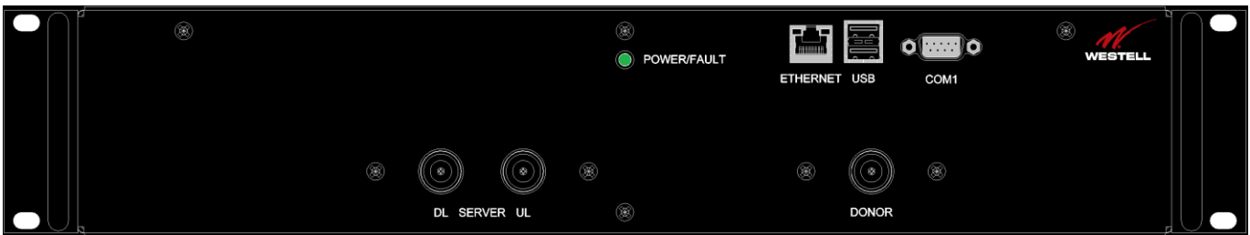
Figure E-17: Single-band D1:S2 Port Configuration
