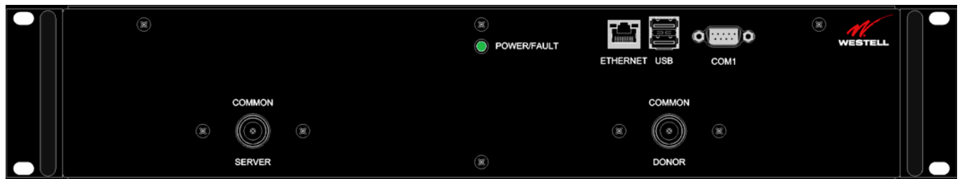
Figure E-12: Dual-band D1:D1 Port Configuration
