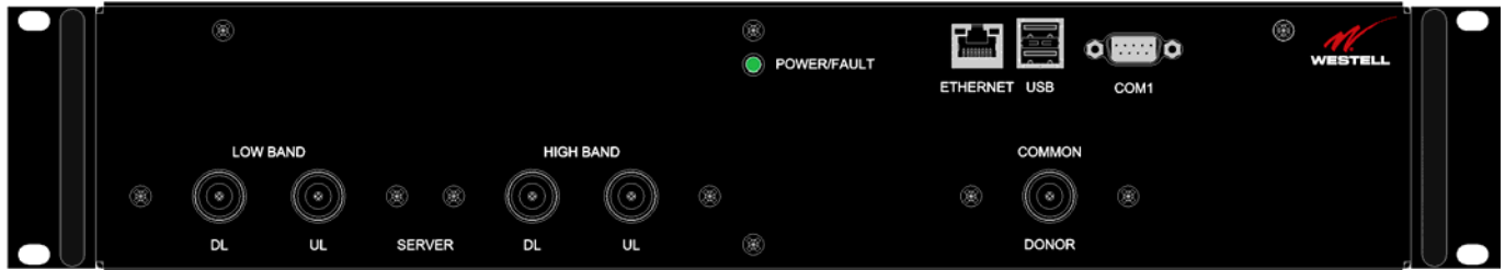
Figure E-16: Dual-band D1:S4 Port Configuration
