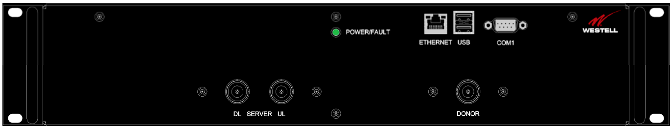
Figure E-17: Single-band D1:S2 Port Configuration
