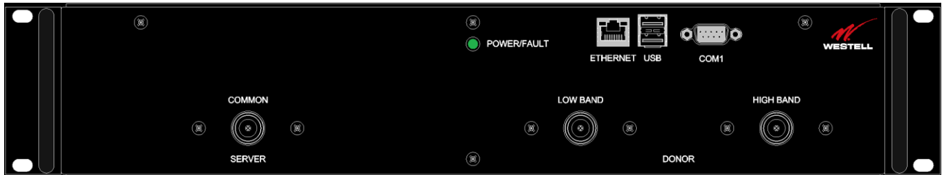
Figure E-9: Dual-band D2:D1 Port Configuration
