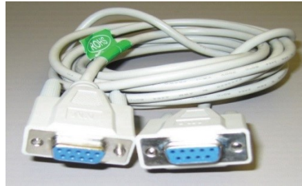
Figure 4-1: Null Modem Cable
