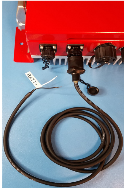
Figure 5-10: Battery Cable Connected to Signal Booster
