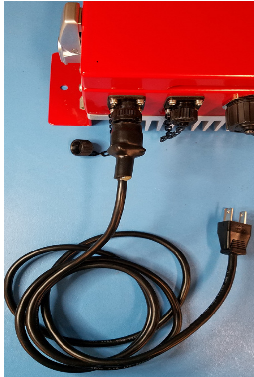
Figure 5-9: Power Cable Connected to Signal Booster
