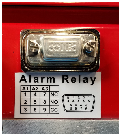
Figure 5-4: Alarm Relay 9 Position D-Sub Connector
