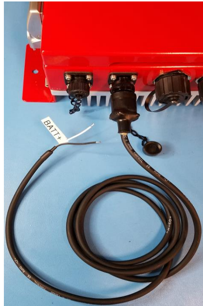
Figure 5-11: Battery Cable Connected to Signal Booster
