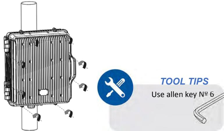
**Figure:** Release Signal Booster cover
