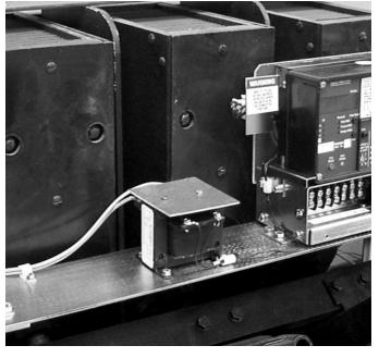
A. Align the holes in the Breaker Mounted CPT with the predrilled holes on the left side of the Trip Unit Mounting Platform. Secure the CPT to the Trip Unit Mounting Platform using the (4) .190-32 × .500" screws, (8) flat washers, (4) lock washers, and (4) nuts supplied. Note that the X1 and X2 terminals face the front of the Breaker.
