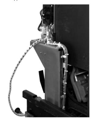
C. Route the Sensor Harness to the bottom of the Sensors. Connect the ring terminals of the Sensor Harness to the Sensors. Refer to Section 12 of the Retrofit Application Data, supplied with the Retrofit Kit, for detailed wiring specifications.
