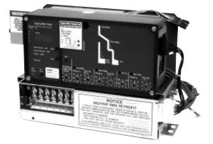
A. For Kits Supplied with a PT Module Only. Mount the PT Module to the Glass Poly Insulation Barrier as shown, using the (2) .138-32 × .500" screws, (4) flat washers, (2) lock washers, and (2) nuts supplied.
