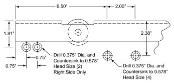
B. Mount the right and left Trip Unit Support Brackets to the Breaker side plates as shown, using the (4) .312-18 × .750" flat head screws, (4) flat washers, (4) lock washers, and (4) nuts supplied. Do not tighten them completely at this time.
