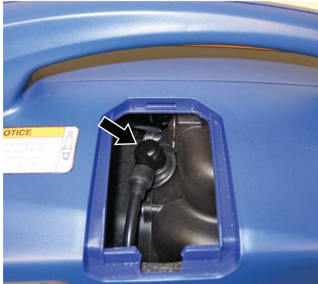
Figure 49 – Removal of Spark Plug Boot (WH1000i Shown)
