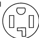
4-Wire Receptacle (14-30R)
