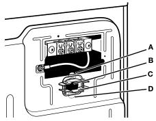
Remove the screws from a ¾" (19 mm) UL listed strain relief (UL marking on strain relief). Put the tabs of the two clamp sections (C) into the hole below the terminal block opening (B) so that one tab is pointing up (A) and the other is pointing down (D), and hold in place. Tighten strain relief screws just enough to hold the two clamp sections (C) together.
