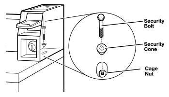
**NOTE:** Installing the security bolt provides added security, but will add to the service time when the top needs to be removed or lifted for servicing the dryer.
