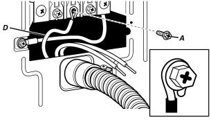
3. Connect remaining wires under outer terminal block screws (F). Squeeze hooked ends together and tighten screws. Finally, reinstall terminal block cover to dryer rear panel. Secure cover with hold-down screw. Now go to "Venting Requirements."
