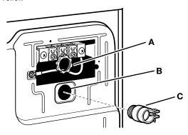
Unscrew the removable conduit connector (A) and any screws from a ¾" (19 mm) UL listed strain relief (UL marking on strain relief). Put the threaded section of the strain relief (C) through the hole below the terminal block opening (B). Reaching inside the terminal block opening, screw the removable conduit connector (A) onto the strain relief threads.
