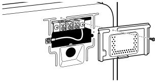
Remove hold-down screw and terminal block cover.
