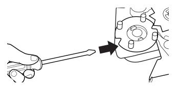
5. Place new cam (hub side down) over clock shaft. Line up flat side of shaft with flat side of cam hole. Check that drive lug is in place.
