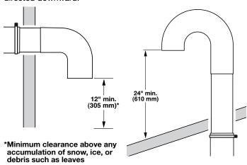
If main vent travels vertically through the roof, rather than through wall, install a 180° sweep elbow on end of vent at least 2 ft. (610 mm) above surface of roof.
