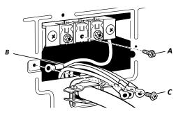
Connect neutral ground wire (B) and neutral wire (white or center wire) (D) of power supply cord under center terminal block screw (A). Tighten screw.
