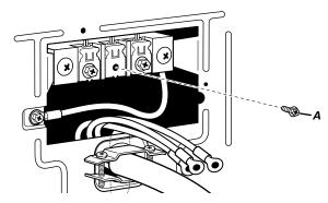
Connect neutral wire (white or center wire) (D) of power supply cord under center terminal block screw (A). Tighten screw.
