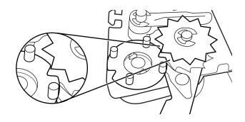
7. Press cam down in place on clock shaft. Make sure that V-shaped notch clears the ratchet tooth.
