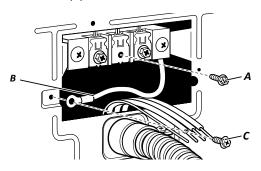
2. Connect neutral ground wire (B) and place hooked end (hook facing right) of neutral wire (white or center wire) (D) of direct wire cable under center terminal block screw (A). Squeeze hooked ends together and tighten screw.
