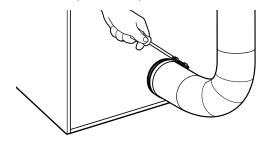
**4.** Make sure the vent is secured to exhaust hood with a 4" (102 mm) clamp.
