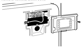
Remove hold-down screw and terminal block cover.
