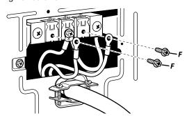
4. Connect a separate copper ground wire (G) under the green external ground conductor screw (C) to an adequate ground. Finally, reinstall terminal block to dryer rear panel. Secure cover with hold-down screw. Now go to "Venting Requirements."
