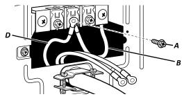
Connect remaining wires under outer terminal block screws (F). Tighten screws.
