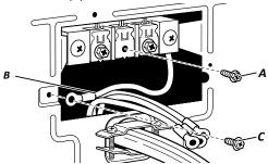
Connect neutral ground wire (B) and neutral wire (white or center wire) (D) of power supply cord/cable under center terminal block screw (A). Tighten screw.
