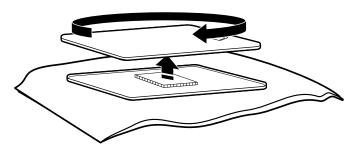
Be certain to keep cardboard spacer centered between doors. Reattach outer door panel to inner door panel so handle is on the side where hinges were just removed.
