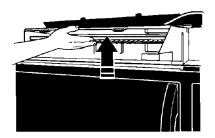
3. Lift the back of the charcoal filter. Slide the filter straight out.
