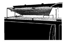
**4. Slide** a new charcoal filter into place. The filter should rest at the angle shown.
