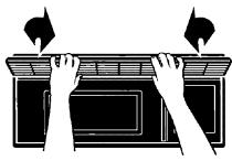
Slide the bottom of the vent cover into place. Push the top until it snaps into place. Replace the mounting screws.
