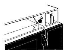
4. Remove bulb holder mounting screw.
