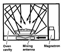
**Microwaves** pass through most glass, paper, and plastics without heating them so food absorbs the energy. Microwaves bounce off metal containers so food does not absorb the energy.
