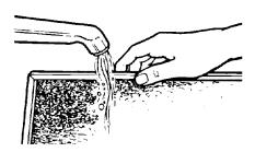
2. Soak grease filters in hot water and a mild detergent. Scrub and swish to remove embedded dirt and grease. Rinse well and shake to dry. Do not clean filters with ammonia, corrosive cleaning agents such as lye-based oven cleaners, or place them in a dishwasher. The filters will turn black or could be damaged.
