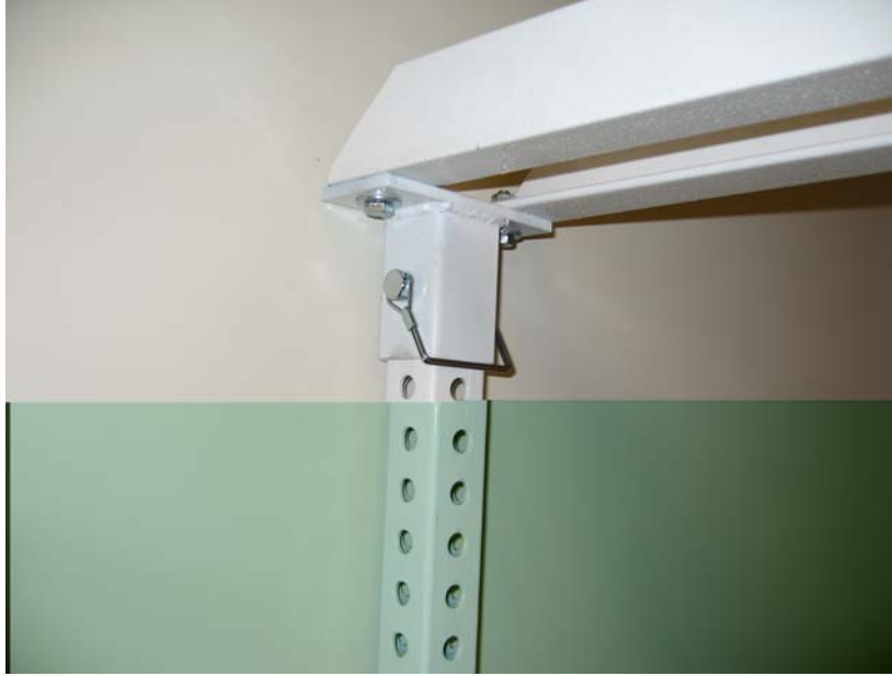
Example of the proper positioning of the leg in the upper assembly and proper pin placement.
