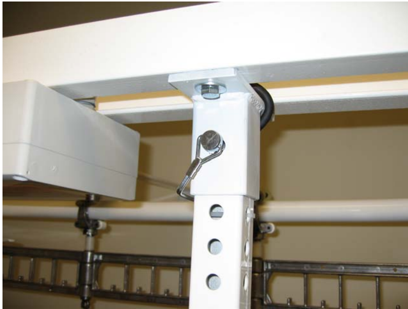
Example of the proper positioning of the leg in the upper assembly and proper pin placement.
