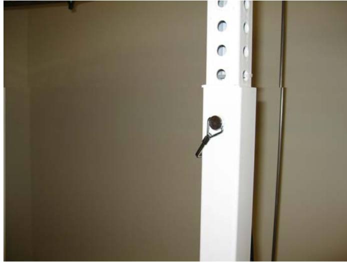
Example: Left Side view of proper locking pin placement
