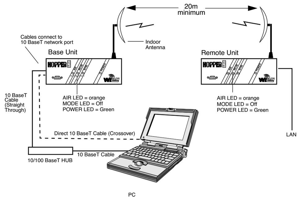
3. Power up each Hopper Plus 120-24 unit. Initially the LEDs should appear as follows:
