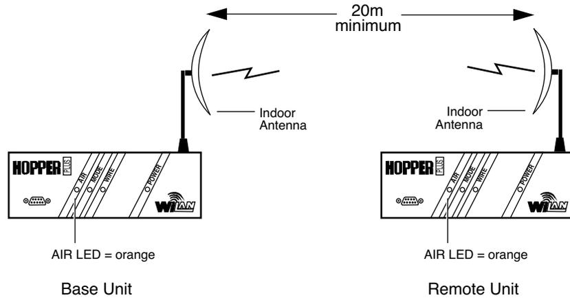
6. Observe the AIR LED of each unit and look for normal status. A normal status is indicated when the AIR LEDs on the base and the remote unit are both orange. The status of the AIR LED is indicated as follows.
