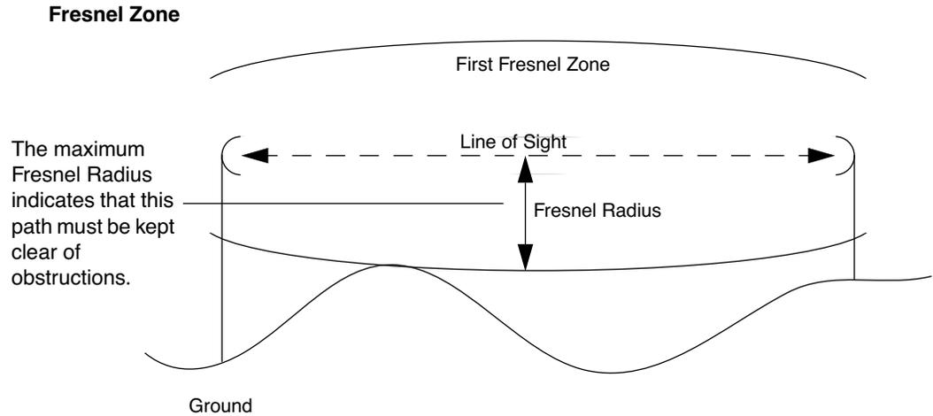
For the 2.4 GHz band, the approximate Fresnel Radius calculated as follows:
