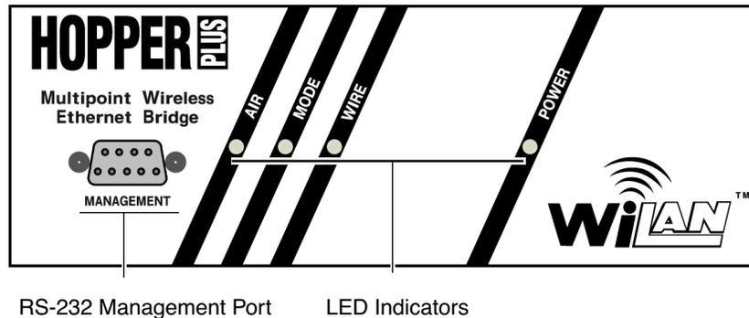
The the front panel connector and LEDs are described below. The color of a LED indicates its status See *Front Panel LEDs*, page 111 for detailed information.
