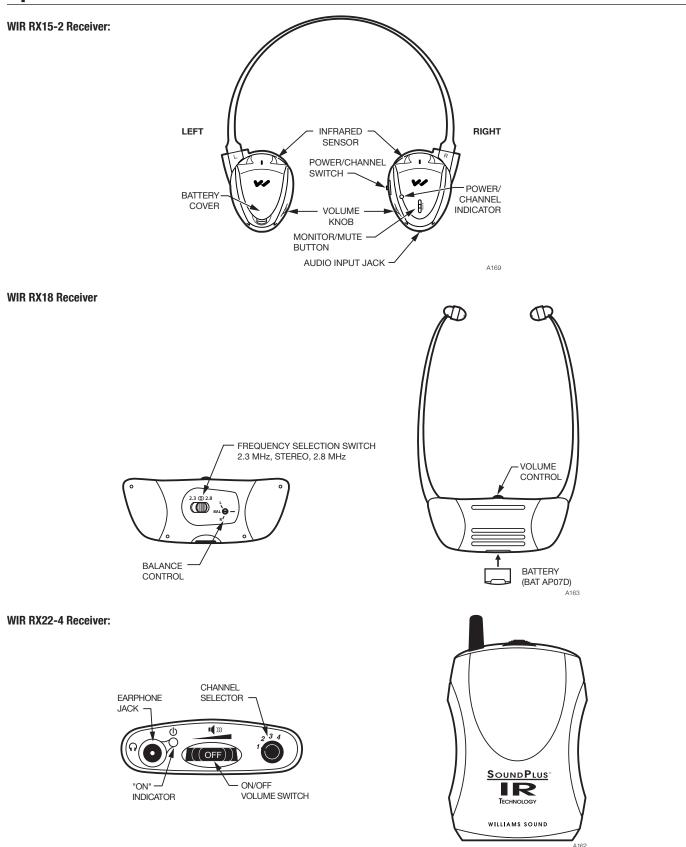
NOTE: On the RX22-4, channel 1=2.3 MHz, channel 2=2.8 MHz, channel 3=3.3 MHz, and channel 4=3.8 MHz.
