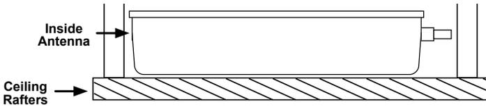
In some cases, multiple Inside Antennas may be required, for instance if you have multiple rooms with poor signal. A signal may be split by using a splitter (sold separately). If using more than one Inside Antenna, a separation of at least 20 feet is necessary between Inside Antennas. See configuration on pages 3 & 4.
