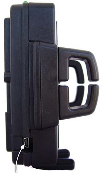
Phone charging connector port. Connect to your phone with optional cables
