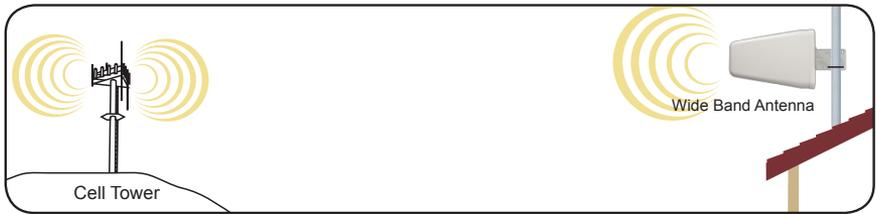
The outside antenna must be mounted at a location outside of the home or building, where the strongest cell signal is present. This can be accomplished by using the Wilson Signal Meter. Alternatively, a cell phone in test mode can be used for finding the area around the building with the strongest signal.
