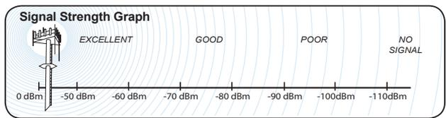
Signal readings usually appear as a negative number (for example, -86). The closer the number to zero, the stronger the signal (see Signal Srength Graph above).
