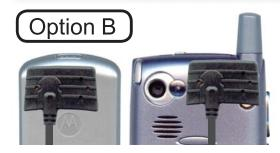
Small Antenna placement is dependant upon the location of the phones antenna. Place the Small Antenna as close as possible to the phones antenna.
