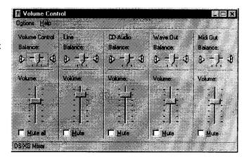
To enable additional (de-select) Playback or Recording Mixer sources, click on Options, then Properties. Check (uncheck) the box associates to the desired device.
