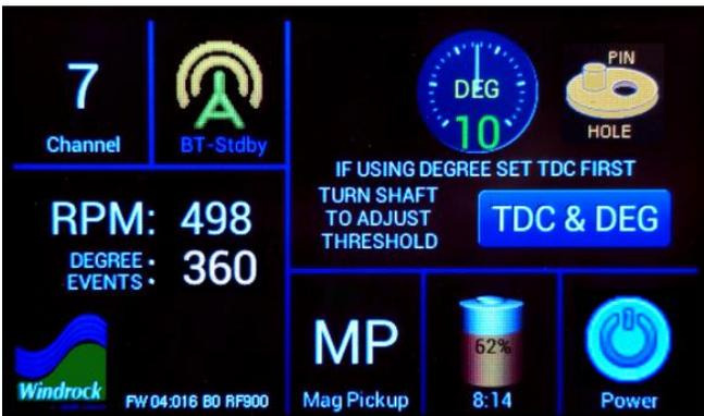
The threshold gage for the DEG pickup is identical to the TDC gauge and should be adjusted in the same way TDC ONLY mode is except that the degree events value is referenced during adjustment rather than RPM.
