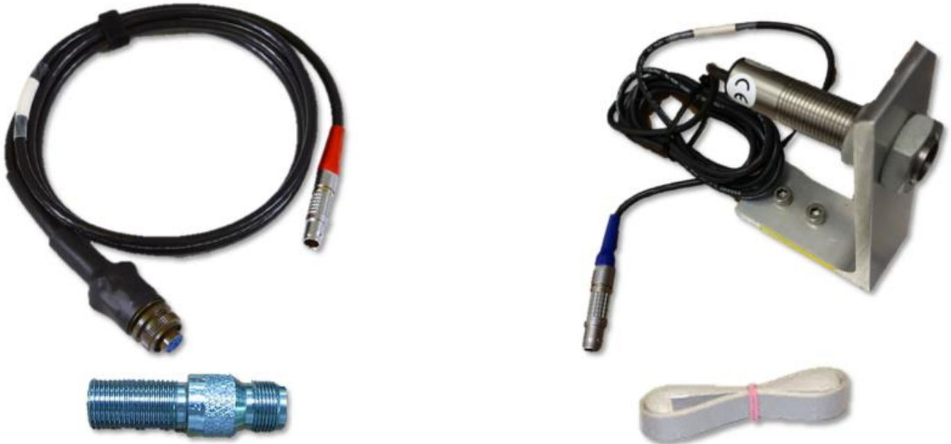
Both of these methods works well to provide a once-per-turn synchronization reference by tracking the revolution of a reflective reference such as a hole, pin or reflective tape.
