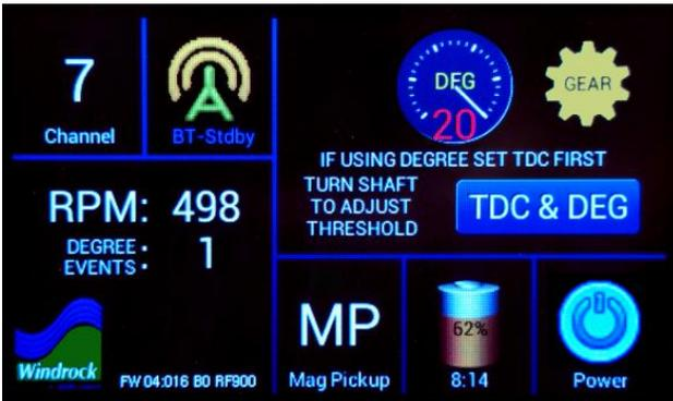
The MP mode can also be configured to add a second magnetic pickup for detecting degree signals by pressing the **TDC ONLY** / **TDC & DEG** button which toggles between TDC only mode and TDC & DEG mode.
