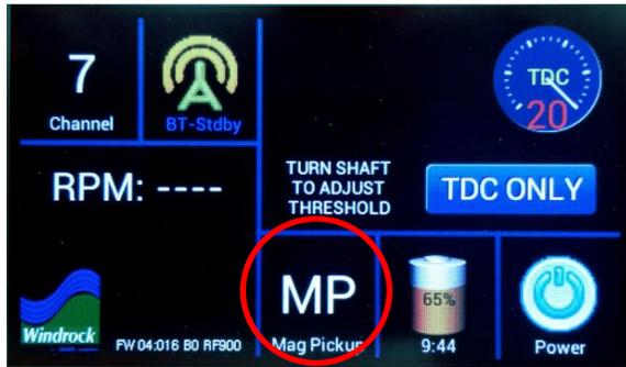
The threshold adjustment controls the sensitivity or level detection of the signal. It defaults to 20 (least sensitivity) and can be adjusted up or down by slowly rotating the shaft.
