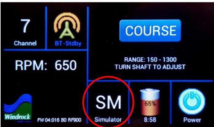
It is possible to use the timing light in this mode to estimate speed on pumps/fans and collect crank angle data where a speed reference is not available. The range of this feature is 150-1300 RPM. The COURSE / FINE toggle button allows for course / fine adjustment in the RPM value.
