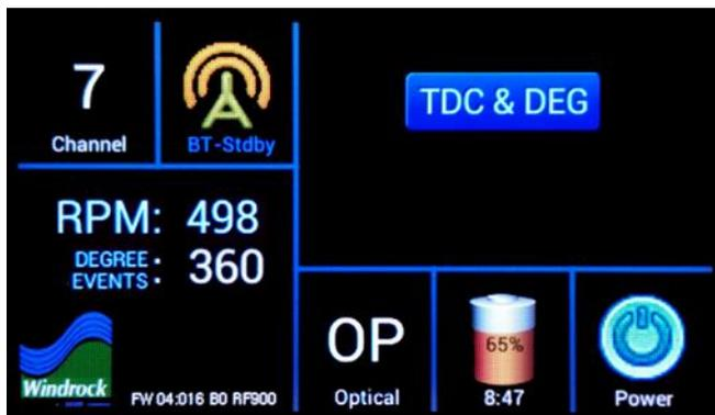
Like the MP mode, this mode also has a **TDC ONLY** / **TDC & DEG** button which toggles between TDC only mode and TDC & DEG mode.
