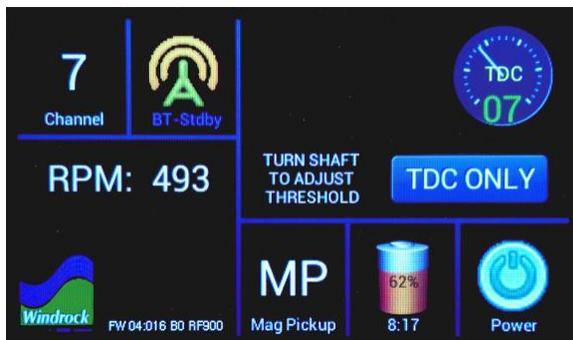
Once the signal level exceeds the threshold level, the device will calculate an RPM and display it if the RPM is within measuring range as shown.
