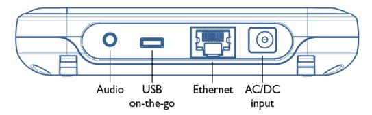
The SimPad may be powered from the mains using the supplied AC/DC adaptor. Plug it in to the appropriate AC/DC input connector.
