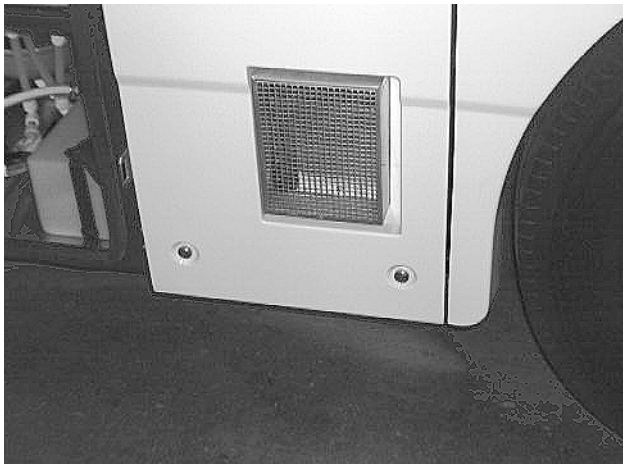
Water Heater Service Access Panel
