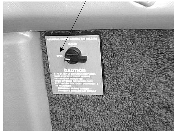
Emergency Position - Open (Normal - Closed)
