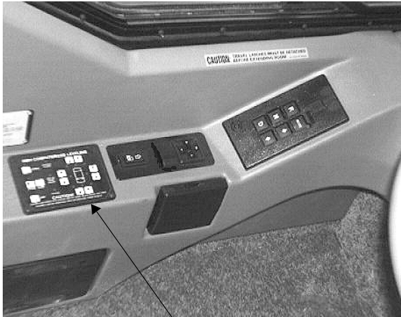
Automatic Leveling System Control Panel
