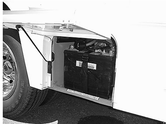
House Battery Compartment Models 22E & 22R (also 24F diesel chassis option)
