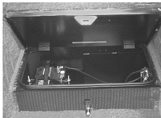
House Battery Storage in Entrance Step Models 24F, 24V, 26A, 27L, 29B, 29K, 31C & 32G (chassis batteries for 24F diesel chassis option)
