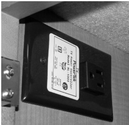
Front TV Ignition Switch Interlock -Typical View
