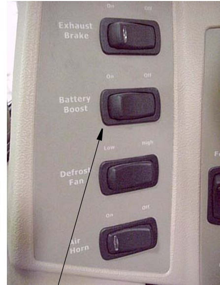
Battery Boost Switch
