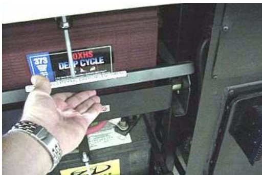
Lift Battery Tray Retainer Latches
