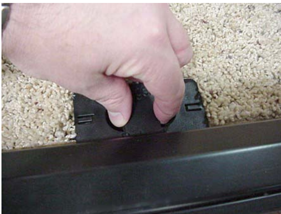
Lift snap-in plate from front edge of step cover.
