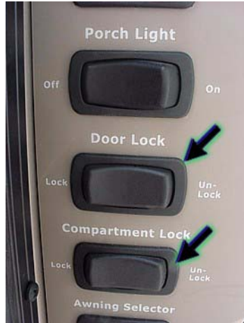
Power Door Locks on entry switch panel
