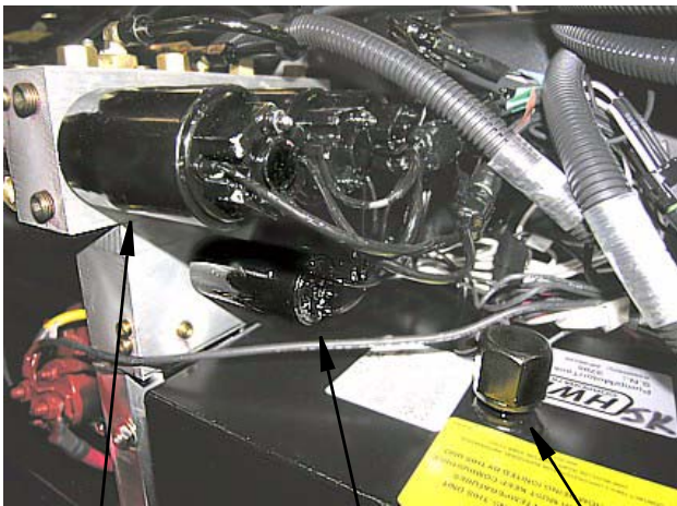
Leveling Jack Valves (Larger) Slideout Room Valves (Smaller) Hydraulic Oil Fill Cap
