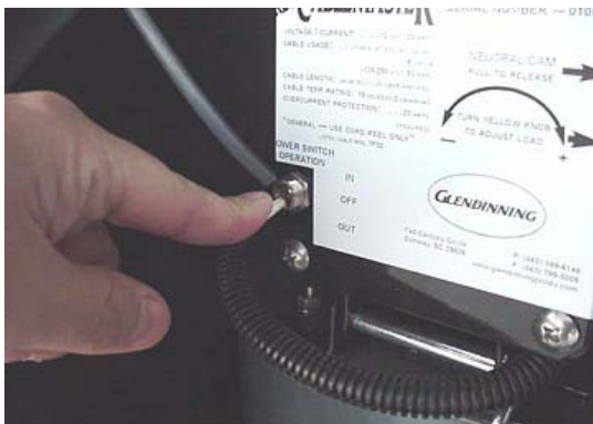
Press and hold switch to extend or retract power cord
